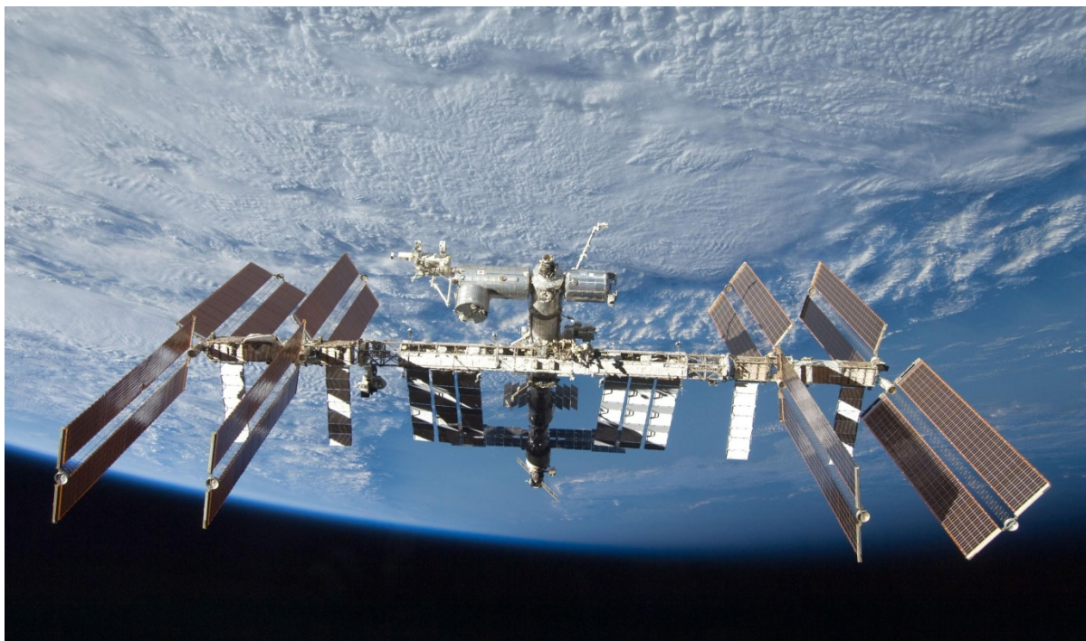
Figure 6: The International Space Station (ISS) in orbit. It is around 100 m in length, not much less than the 112 m diameter required for a 4 rpm space settlement. The mass of the ISS is about 0.42 kT [NASA 2015], or about 5-20 x less than the 4 rpm versions of the Stanford Torus and Kalpana One (see Tables 2 and 3). The ISS has hosted 7 paying tourists. Image credit: NASA.
